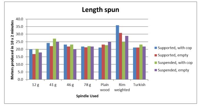
The soapstone spindles all rotated at roughly 13 - 18 Hz under the various conditions, as did the plain and rim-weighted wooden spindles. The Turkish spindle was significantly slower.
